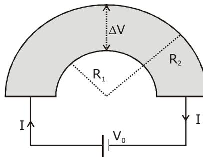
(A)  $I = \frac{V_0 t}{\pi \rho} \ln\left(\frac{R_2}{R_1}\right)$
